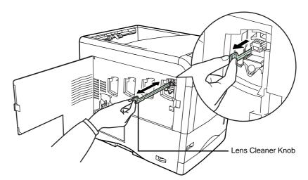
2 Push the lens cleaner knob back in completely. After cleaning, make sure you restore the lens cleaner knob to its home position.
